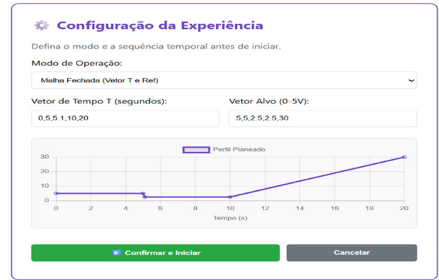
Figure 1 - Dynamic experiment configuration interface, allowing the definition of Time ( T ) and Reference ( Ref ) vectors with a real-time preview of the planned signal profile.
